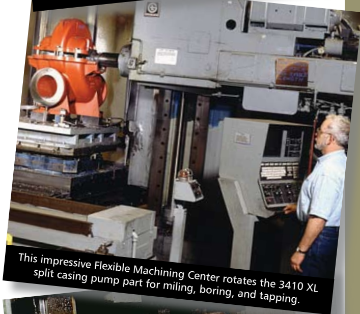
Sophisticated CNC Boring holds tolerances to the most stringent industrial standards.
