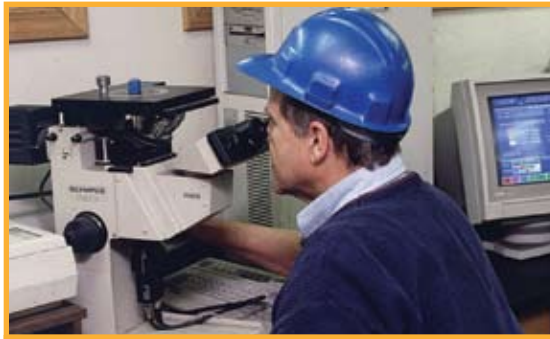
The Foundry's lab technician performs daily audit functions such as checking sand strength - a critical process in the making of molds. The metallurgist is checking the microstructure of metal.
