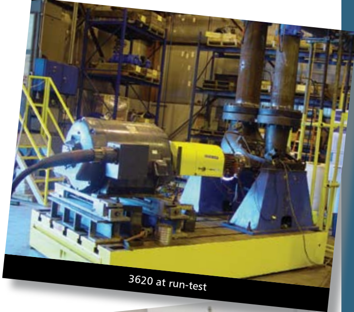
A performance test of the model 3620 API pump is run to confirm that flow conditions and efficiencies are within customer specification.
