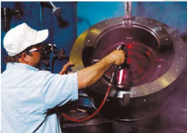
This liquid penetrant test, performed on a Model 3620 casing head to assure structural conformance, is an example of the EPO's non-destructive examination capabilities.
