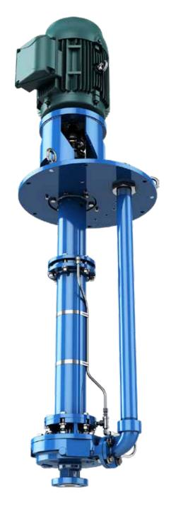
The LF3171 is specifically designed to provide superior performance for low flow flow high head sump applications. Its concentric (circular volute) casing and open radial vane impeller are designed to eliminate hydraulic and mechanical problems at throttled low flows. Radial loads are reduced as much as 85% versus standard volutes at low flows.
