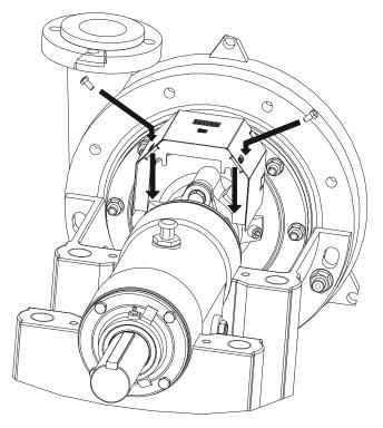
Figure 26: Shaft guard assembly
