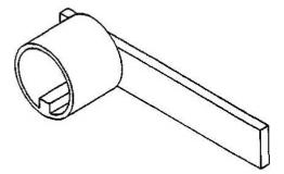
Figure 21: Shaft rotator to install and remove the impeller from the casing
