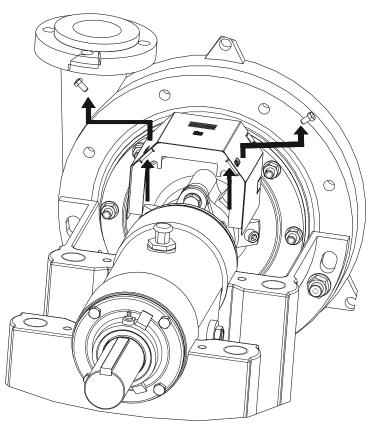
Figure 24: Shaft guard removal
