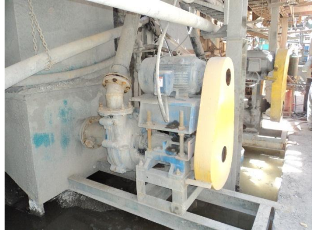
The Goulds 125 XHD pump on mill discharge duty. The competitor's 8x6-18 pump can be seen in the background.
